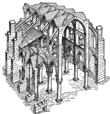
FIG. 105.—CONSTRUCTIVE SYSTEM OF GOTHIC CHURCH, ILLUSTRATING PRINCIPLES OF ISOLATED SUPPORTS AND BUTTRESSING.
