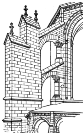
FIG. 107.—EARLY GOTHIC FLYING BUTTRESS.
