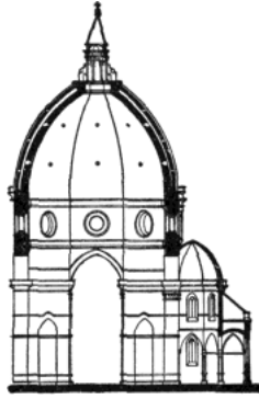
FIG. 159.—SECTION OF DOME OF DUOMO, FLORENCE.
